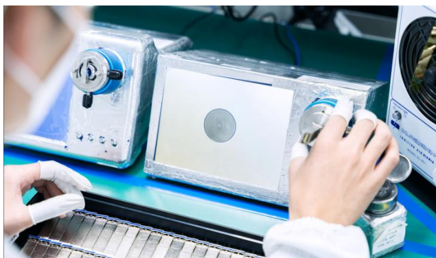
Optical endface inspection
